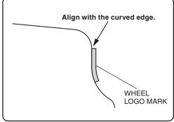
3. Partly remove the adhesive backing from behind the wheel logo mark.
