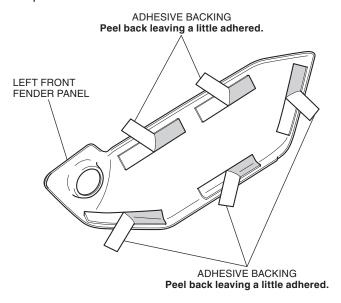
4. Attach the left front fender panel as shown.
