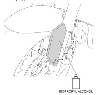
3. Peel off the adhesive backing on the left front fender panel as shown.
