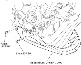
15. Tighten the screws as shown.
