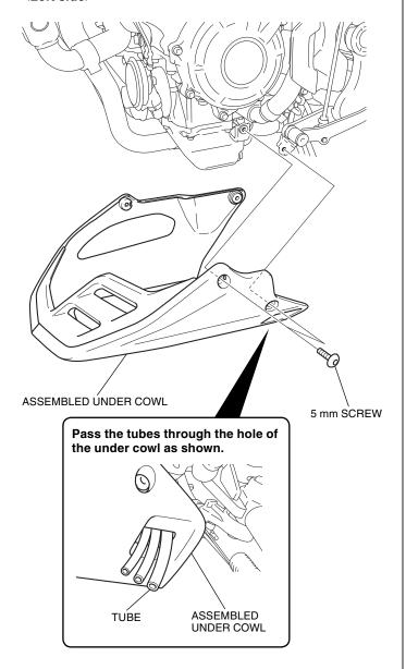
14. Loosely install the screws as shown.
