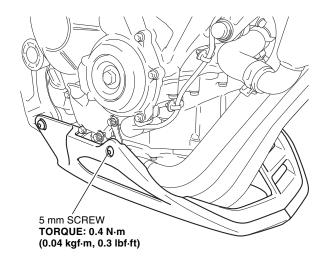
16. Tighten all loosely installed hardware to the specifications in the torque chart.
