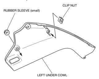
9. Install the clip nut and rubber sleeve as shown.
