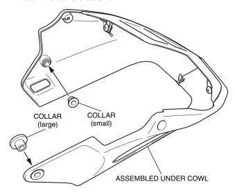
13. Loosely install the assembled under cowl as shown. **<Left side>**
