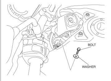
6. Remove the indicated parts with raising the front part of the fuel tank.
