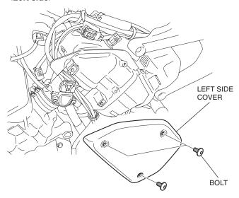
10. Remove the bolt as shown. **Left side>**
