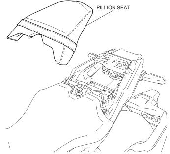
2. Remove the main seat and disconnect the negative (-) cable of the battery.
