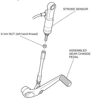
15. Install the gear change arm as shown.
