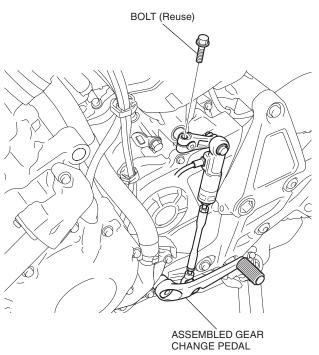
21. Tighten the loosely installed parts securely to the dimension shown.
