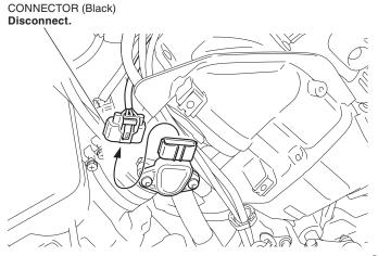
24. Disconnect the dummy connector as shown.
