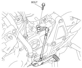
11. Remove the gear change pedal as shown.
