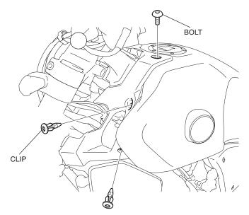
4. Remove the tank front cover as shown.
