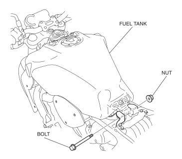
8. Remove the fuel tank as shown.
