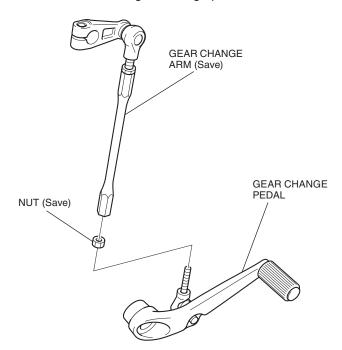
13. Loosely install the change bar and gear change pedal as shown.
