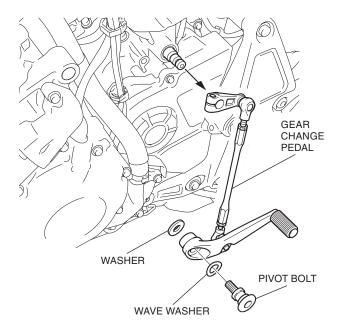
12. Disassemble the gear change pedal as shown.
