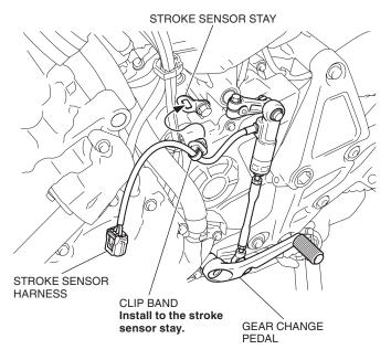
23. Disconnect the connector as shown.
