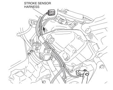
26. Connect the stroke sensor harness as shown.
